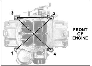
Figure 4—Carburetor hold-down nut torque sequence
